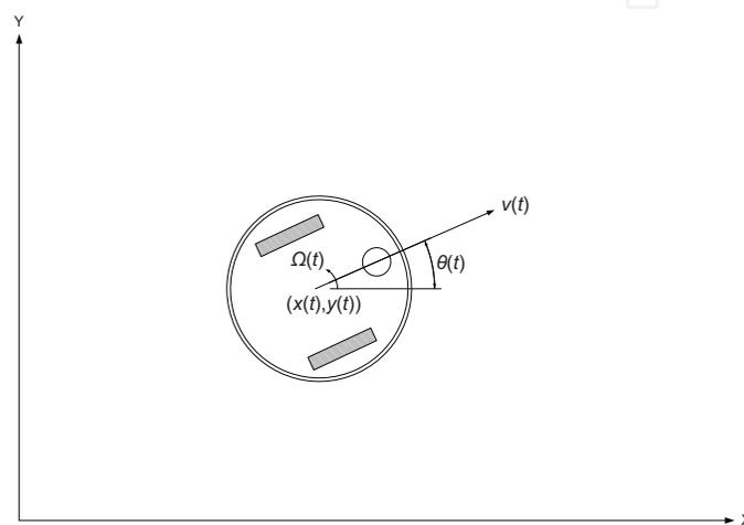
Fig. 3. Kinematic Model of Individual Robot
