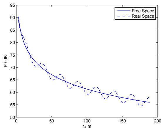
Fig. 6. Log-Normal Signal Loss Distribution
