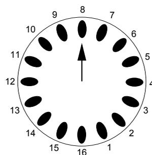
Fig. 2. Proximity Sensor System of Individual Robot
