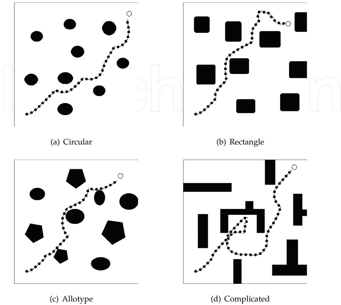
Fig. 13. Single Robot Move to the Potential Target with Path Planning
