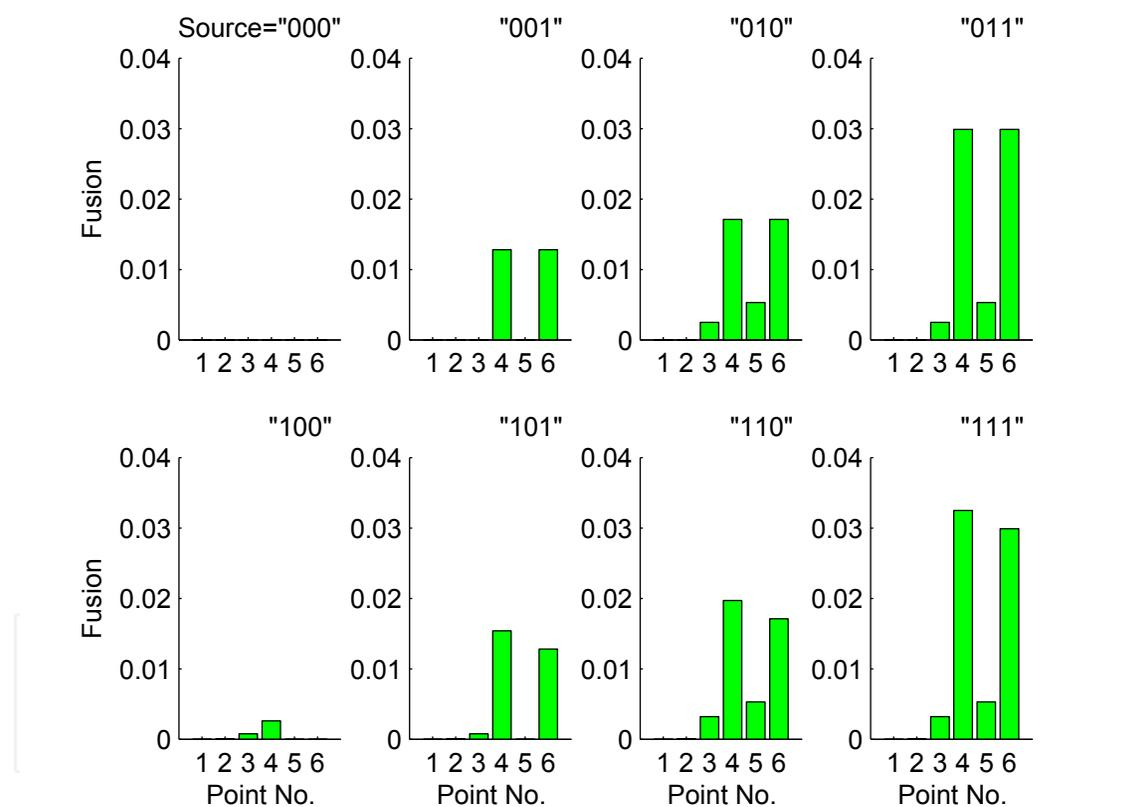
Fig. 11. Fusion results at the assigned six measuring points under different encodes of information source. Note that the title *Source*="000" of the left corner sub-figure represents no GAS, no RF, and no CALL signals are emitted when sampling. One can understand the other cases in a similar manner. Besides, the fusion is a scalar value without any physical meaning.
