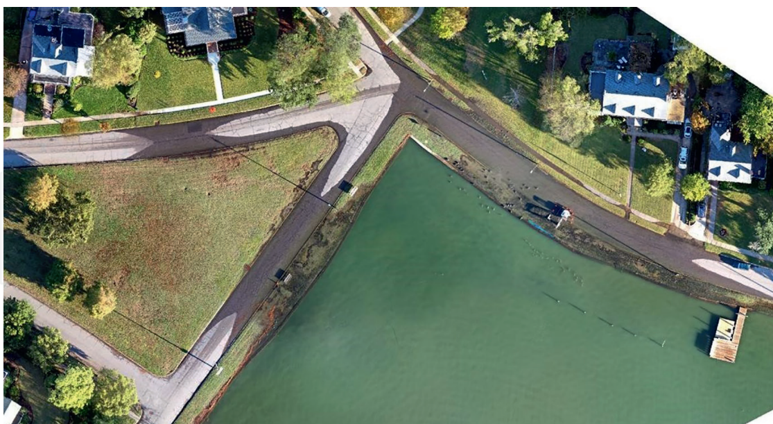
Figure 8. King tide flooding in the Larchmont neighborhood of Norfolk, Virginia, is captured by wetted surfaces just after high tide in this UAV orthomosaic mosaic (October 29, 2019). Such flood footprint mapping provides for the validation of numerical hydrodynamic models and operational flood forecasts.
