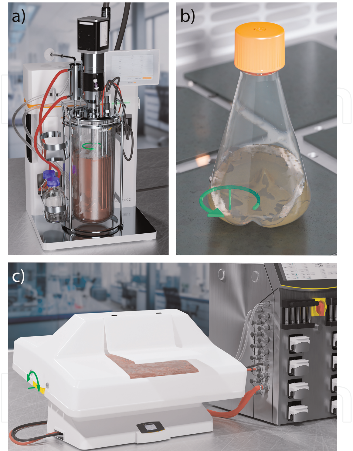
Figure 1. Computer-generated images (CGI) of common mechanically driven bioreactor systems. a) Stirred bioreactor where the power is brought into the system by rotation of the stirring shaft and the stirrer (rotation marked by green arrow). b) Shake flask, which is an orbitally shaken bioreactor. Here the power is brought into the system by the orbitally shaking of the platform (movement of the platform marked by green arrow). c) Wave-mixed bioreactor, in which the power is brought in by the back and forth tilting of the bioreactor (rotation around tilting axis marked by green arrow).
