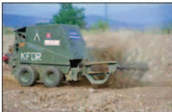
Fig. 1. The remotely operated flailing vehicle „Božena 1”
