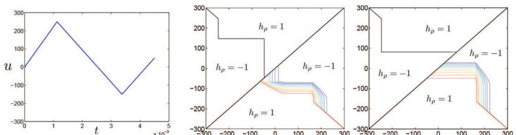
**Figure 7.** Input function  $u(t)$  (left) defined in  $[0, 0.0045]$ . The isolines represent the corresponding dynamic relay values  $\eta_\rho$  with  $k = 50$  and the classical relay  $h_\rho$ , at  $t = 0.003$  (center) and  $t = 0.0045$  (right).
