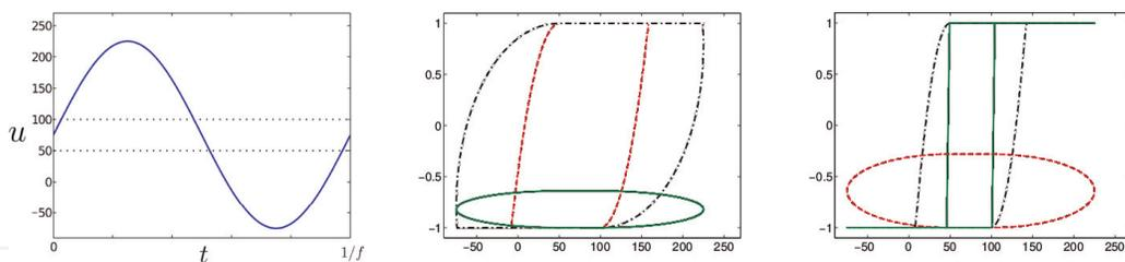
**Figure 6.** On the left panel, input function  $u(t) = 150 \sin(2\pi ft) + 75$ . The center graph shows the  $(u, y)$  curve corresponding to the dynamic relays with  $k = 50$  and initial state  $\xi = -1$  for frequencies  $f=50, 500, 5000$  Hz (dashed, dash-dotted and solid line, respectively). On the right panel, the  $(u, y)$  curve is depicted for  $f= 5000$  Hz and  $k = 10^2, 10^4, 10^8$  (dash-dotted, dashed and solid line), respectively.
