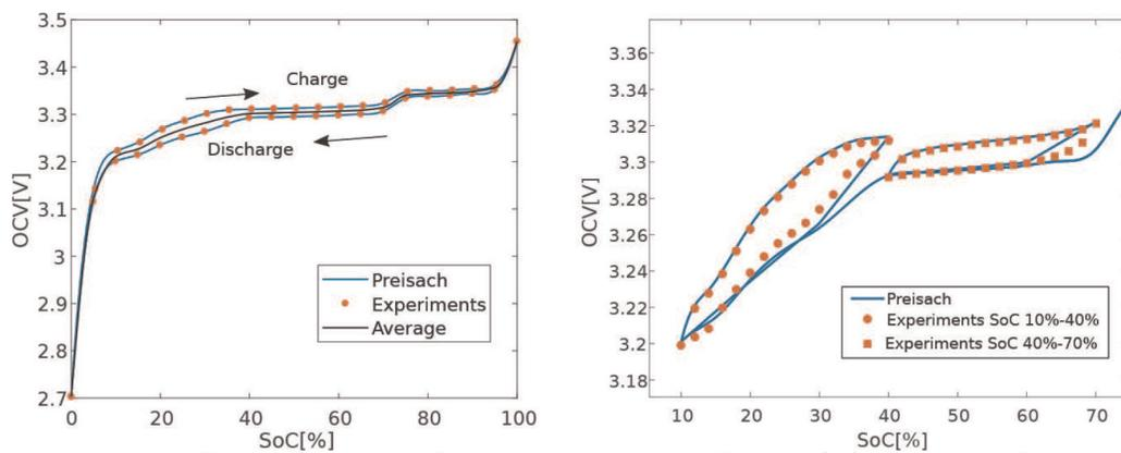
**Figure 12.** Measurements along the major loop and the approximation given by the Preisach model (left). Experimental inner loops and approximation of the Preisach model for different SoC values (right).
