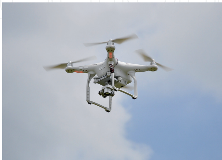
Figure 8. Four-rotor Phantom 2 Vision+ UAV equipped with a high-resolution digit RGB camera used in this study.
