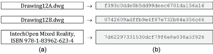
Figure 4. Using MD5 hash function for irreversible data encryption.
