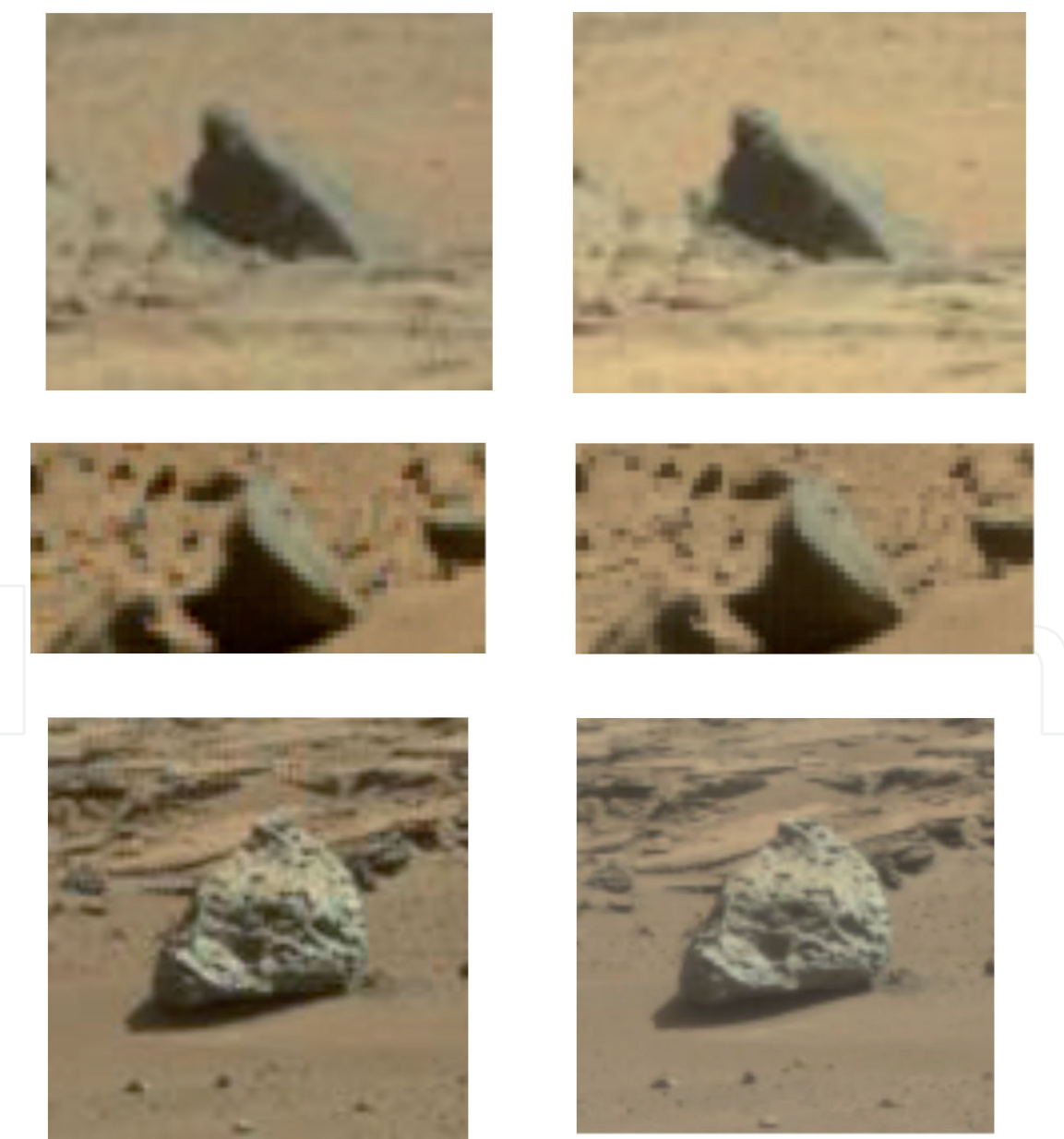
Figure 3. Comparative of demosaicing images. Left column: NASA’s existing software; right column: State-of-the-art deep learning approach.
