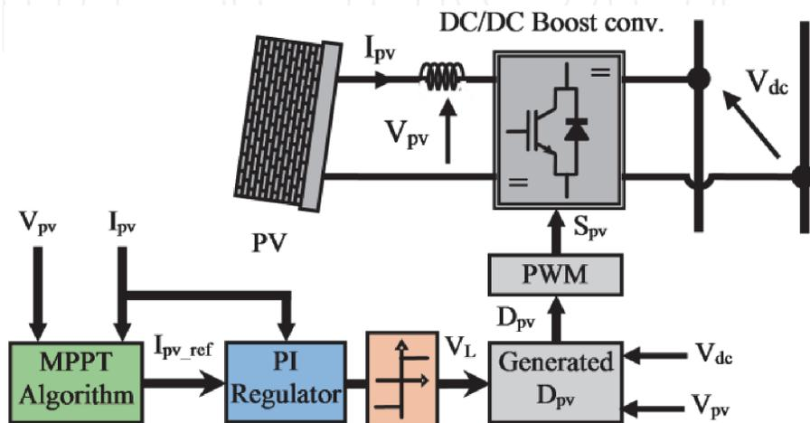
**Figure 5.** MPPT algorithm control scheme of PV array.
