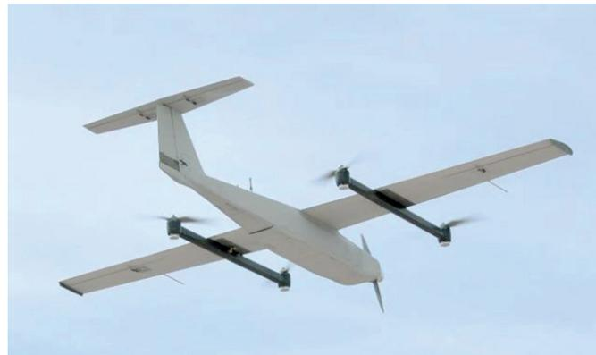
Figure 4. A hybrid fixed-wing-multi-rotor UAV [9].
