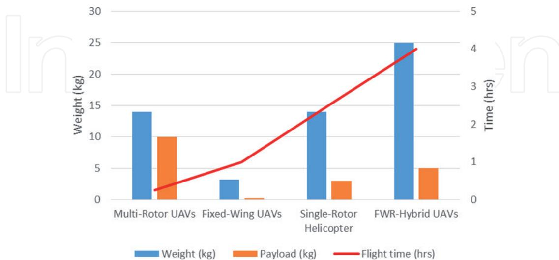
Figure 5. UAV weight and payload vs. flight time.
