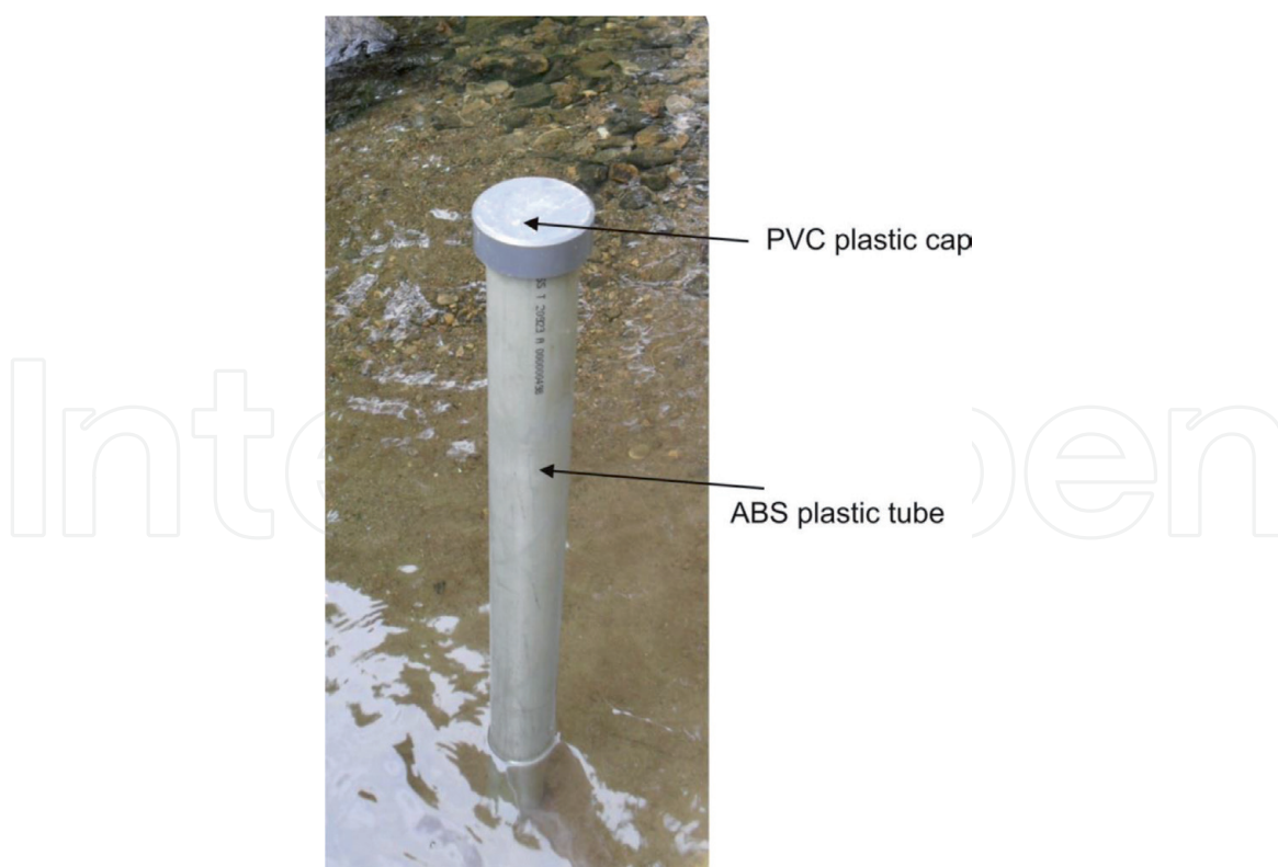
Figure 1. DGT placed in the base of the hollow sampler and left for 24 hours.
