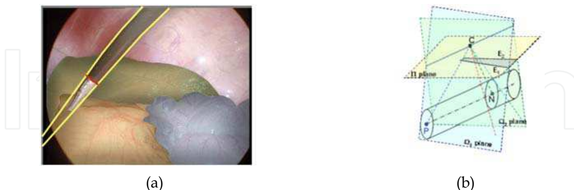
Fig. 8. Video-based tracking of surgical tools (Cano et al., 2008). (a) Image processing for extracting 2D information (b) Model of the laparoscopic tool used for calculate the 3D position and orientation of the tools; C: optical center, P: tip of the tool; N: point of the cylinder axis which projective line is perpendicular to this axis; \Omega_1, \Omega_2 : planes of sight of the tool edges; \Pi plane: image plane; E_1, E_2 : projective tool edges.
