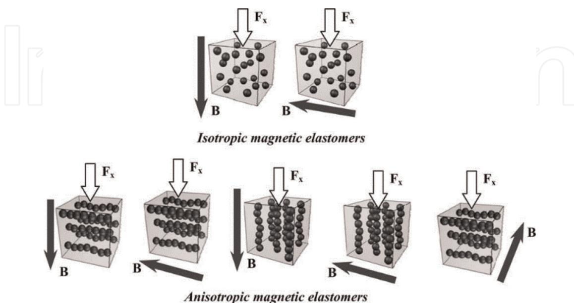
**Figure 9.** The magneto-dependent compressive experiments of MR elastomers with different particle distribution states [80]. The white hollow arrow represents the direction of compressive loading, and the solid black arrow represents the direction of magnetic field.
