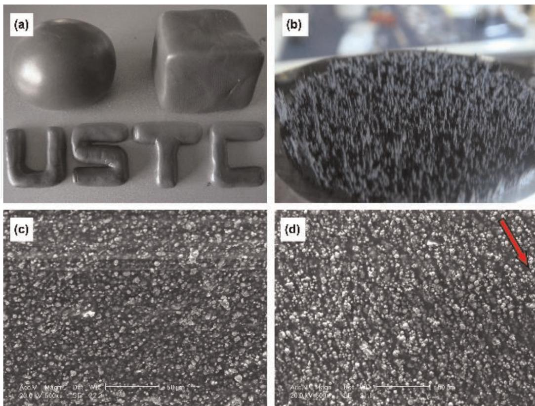
**Figure 4.** The images of MR plastomer without (a) and with (b) magnetic field [58]. The SEM images of MR plastomer without (c) and with (d) magnetic field (the direction of magnetic field is marked by the red arrow) [59].
