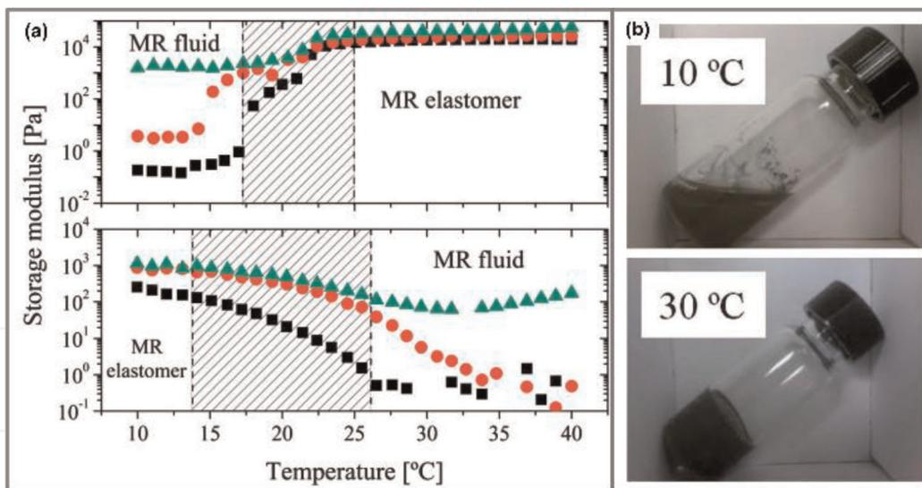
**Figure 6.** Temperature dependent  $G'$  of MR composites with PEO-PPO-PEO copolymer solution (upper subfigure) and P-NIPA microgel dispersion (lower subfigure) (a). Photos of the copolymer-based MR material at different temperatures after 1 h at rest (b) [67].
