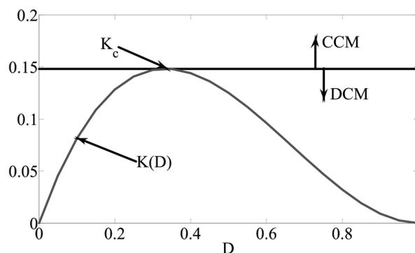
**Figure 5.**  $K(D)$ ,  $K$ , and conduction mode (CM) conditions.
