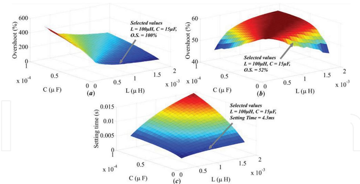
**Figure 10.** (a)  $G_{vd}$  step system response for varying  $L$  and  $C$ : overshoot with zeros. (b)  $G_{iLd}$  step system response for varying  $L$  and  $C$ : overshoot with zeros. (c) Step system response varying  $L$  and  $C$ : setting time.
