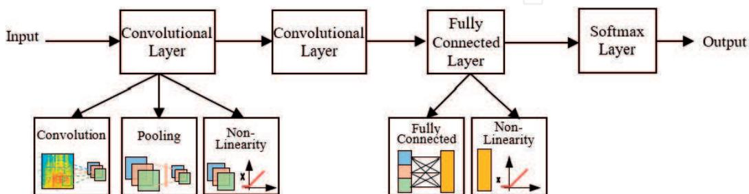
**Figure 5.** Block diagram of convolutional neural network.
