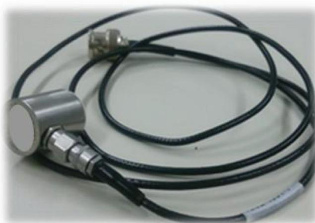
**Figure 3.** A typical AE sensor with connecting cable.
