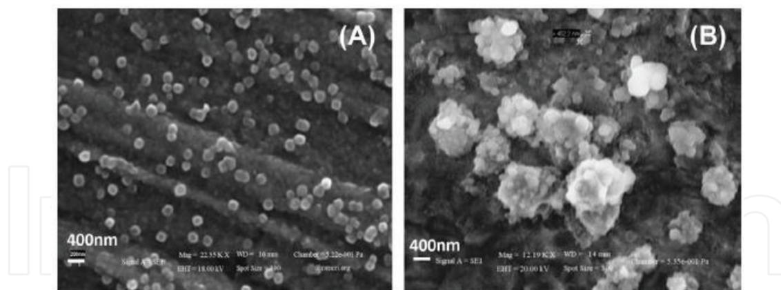
**Figure 5.** SEM images of nanoparticles formed with (A)  $[\text{bmim}^+][\text{C}_8\text{OSO}_3^-]$  and (B)  $[\text{omim}^+][\text{Cl}^-]$ . From Ref. [43] with permission of Elsevier Limited.
