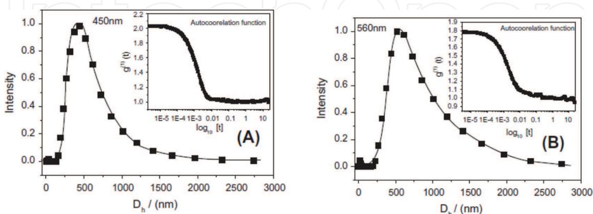
**Figure 4.** Hydrodynamic diameter (D<sub>h</sub>) plots of chitosan nanoparticles formed with (A) [bmim<sup>+</sup>][C<sub>8</sub>OSO<sub>3</sub><sup>-</sup>] and (B) [omim<sup>+</sup>][Cl<sup>-</sup>]. From Ref. [43] with permission of Elsevier Limited.
