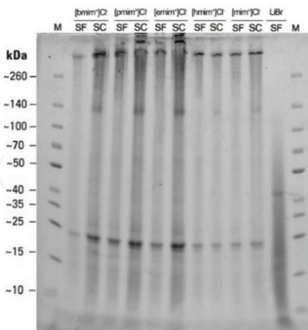
**Figure 6.** Sodium dodecyl sulfate-polyacrylamide gel electrophoresis of the protein components of silk fibroin (SF) and white silk cocoons (SC) after the use of high-power ultrasounds in the solutions SC/IL or SF/IL with ILs: [bmim<sup>+</sup>][Cl<sup>-</sup>], [pmim<sup>+</sup>][Cl<sup>-</sup>], [emim<sup>+</sup>][Cl<sup>-</sup>], [hmim<sup>+</sup>][Cl<sup>-</sup>] and [mim<sup>+</sup>][Cl<sup>-</sup>]. From Ref. [23] with permission of Wiley Online Library.
