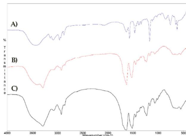
**Figure 8.** Comparative FTIR spectra of (A) only [bmim<sup>+</sup>][Cl<sup>-</sup>]; (B) SFNs regenerated from SF/[bmim<sup>+</sup>][Cl<sup>-</sup>] solution; (C) SFNs regenerated from classical CaCl<sub>2</sub>/EtOH/H<sub>2</sub>O solution [52]. From Ref. [23] with permission of Wiley Online Library.
