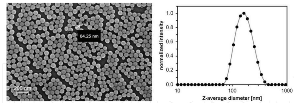
**Figure 3.** (left) Scanning electron microscopy images of nanoparticles obtained by dialysis of xylan phenyl carbonate XPC 20. (right) Size distribution of XPC 20 nanoparticles obtained by dynamic light scattering. From Ref. [31] with permission of Elsevier Limited.
