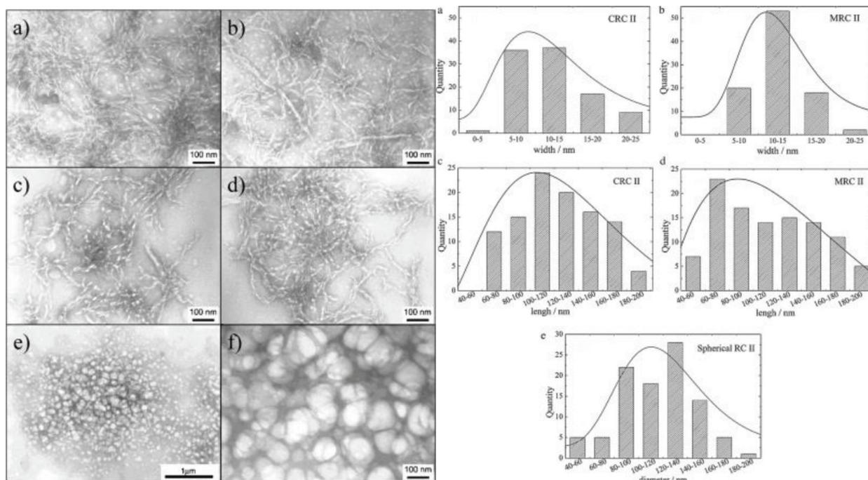
**Figure 1.** (Left) TEM images of MCC-NP (a), CC-NP (b), homogenized MCC-NP (c), homogenized CC-NP (d), and spherical NP from MCC (e, f). (Right) The dimension distribution of homogenized CC-NP, MCC-NP, and spherical MCC-NP. (a) and (b) width distribution of C-RCNs and M-RCNs; (c) and (d) length distribution of C-RCNs and M-RCNs; (e) diameter distribution of spherical RCNs. From Ref. [27] with permission of Elsevier Limited.
