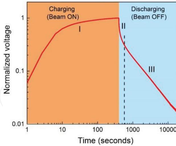
**Figure 3.** Representative charge/discharge curve of PI material bombarded with a non-penetrating electron. Shaded areas represent the three regions of the charge/discharge curve. See text for further details.
