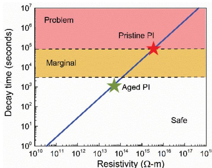
**Figure 2.** The plot of charge decay time versus resistivity value for PI. The red star indicates the resistivity of pristine PI and the green star that of laboratory-aged Kapton-H<sup>®</sup>. Figure adapted from [19].
