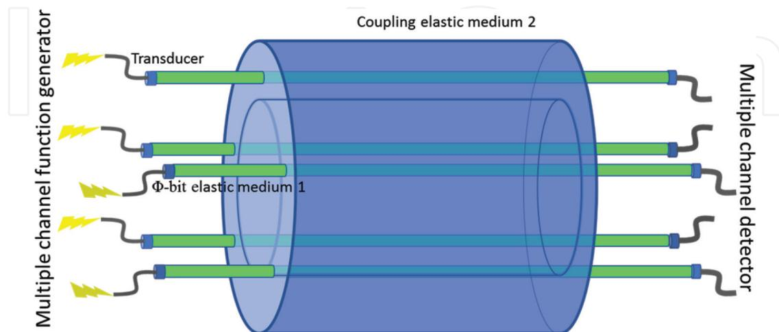
**Figure 3.** Schematic illustration of a five waveguide system. The waveguides are composed of an elastic medium 1 in which mass density and elastic stiffness determine the physical parameter  $\beta$ . The waveguides are embedded in an elastic medium 2 in which mass density and stiffness relate to the parameter  $\alpha$ . The waveguides are actuated via transducers (see the text for details).
