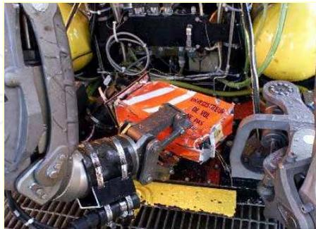
Fig. 4. black-box recovery using ROV, form U.S. Dept. of Defence.
