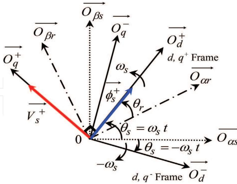
Figure 5. Stator flux orientation under unbalanced grid.
