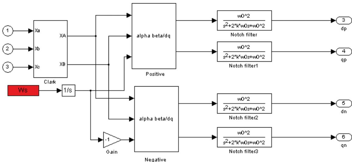
Figure 2. Simulink block for the notch filter method.
