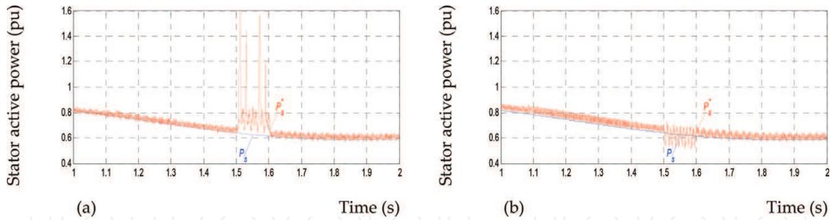
Figure 8. Stator active power (pu): (a) conventional single RCS, (b) proposed dual RCS.
