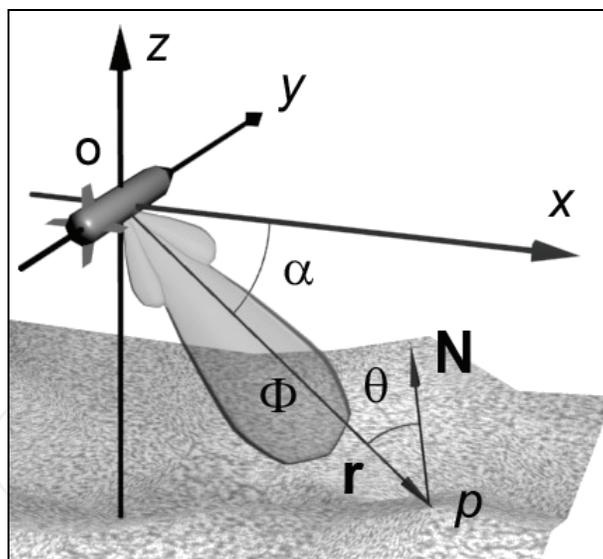
Fig. 4. Side-looking sonar imaging geometry (adapted from (Coiras 2007)).
