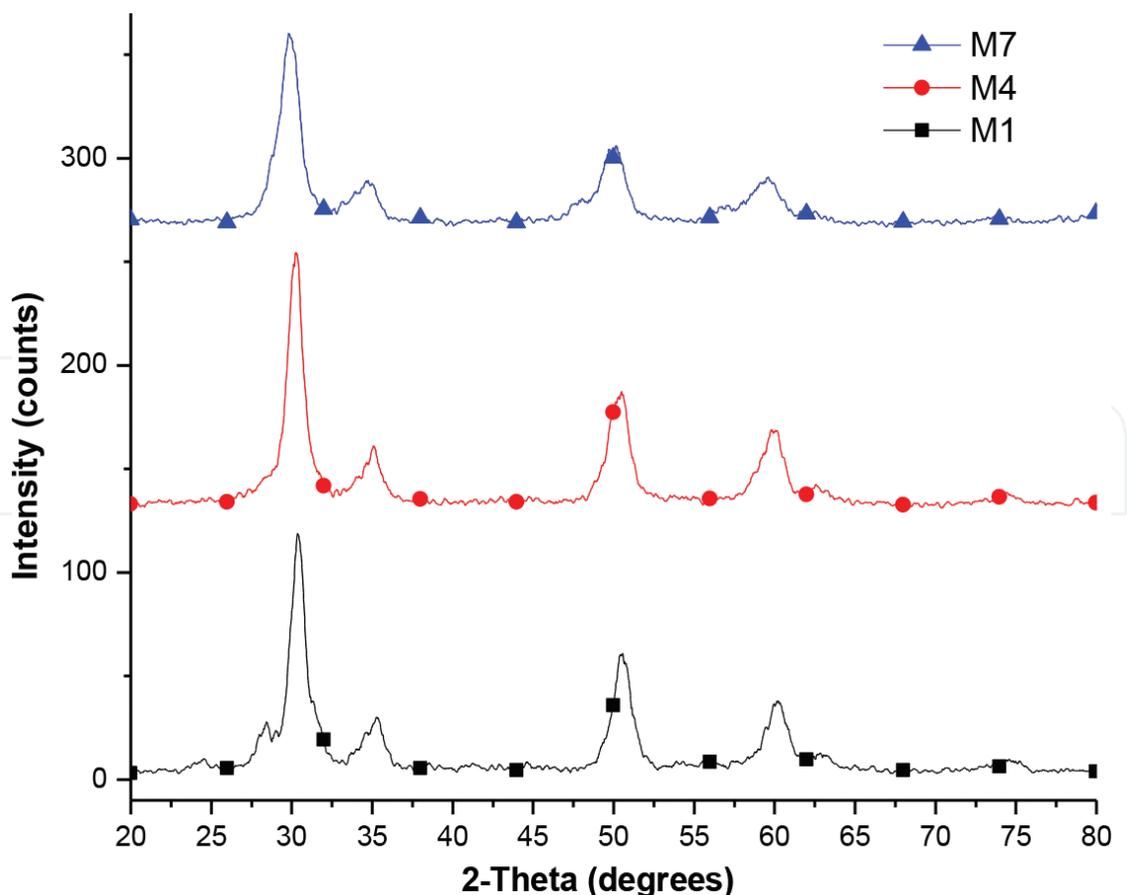
**Figure 2.** X-ray diffraction of M1, M4 and M7, monometallic catalysts.
