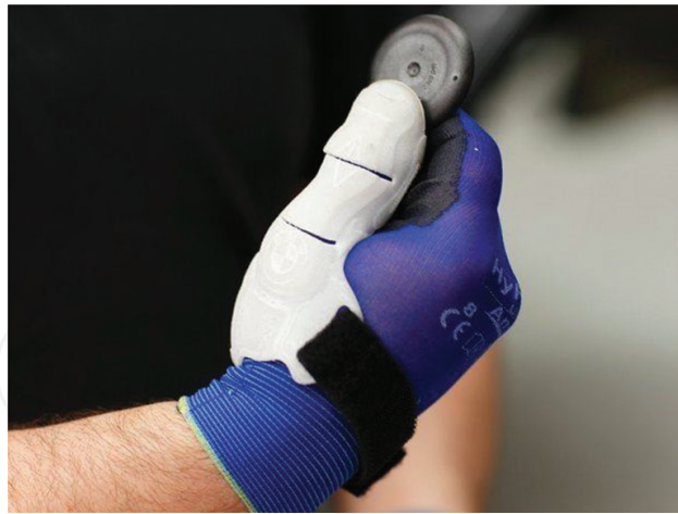
Figure 7. BMW has turned to 3D printing to augment its workers and stop strain on limbs frequently found on manufacturing lines. Photograph: BMW (republished from the Guardian).
