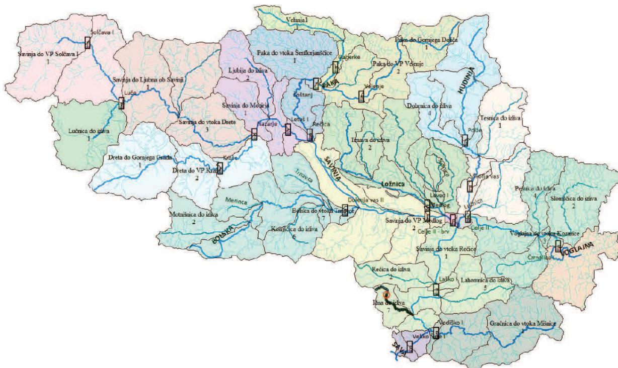
Figure 6. Hydrological model scheme of the Savinja River catchment with 77 sub-catchments.
