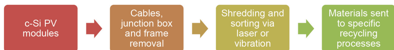
Figure 4. Summary of PV cycle recycling process for c-Si modules [25].
