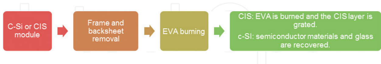
Figure 8. Summary of NEDO recycling process for Si modules (pilot project).
