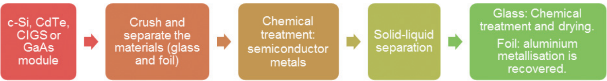
Figure 10. Summary of loser Chemie recycling process for PV modules (pilot project).
