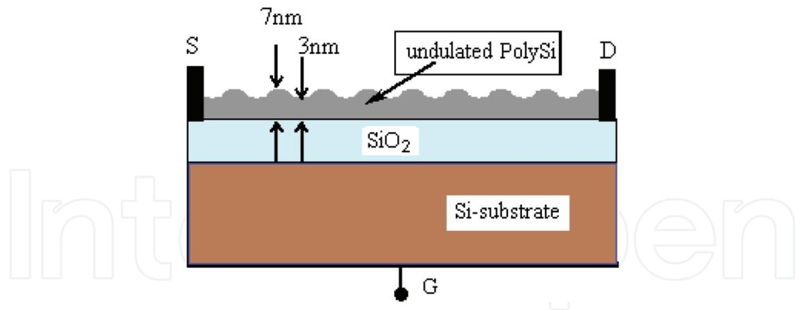
**Figure 1.** A manufactured SOI nanotransistor with maximum 7 nm.
