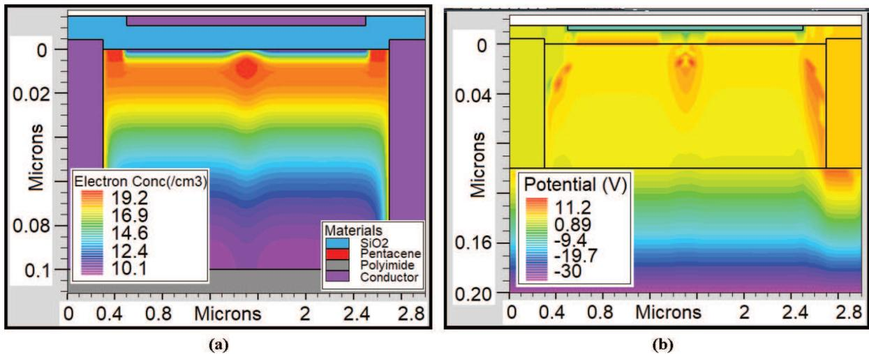
**Figure 3.** (a) The simulation results of a OTFT biased at  $V_s = 0$  V,  $V_D = 40$  V,  $V_{TC} = -10$  V and  $V_{BG} \leq 0$  V, emphasizing the conduction by a volume electron conduction channel; (b) the potential distribution in OTFT biased at  $V_s = 0$  V,  $V_D = 4$  V,  $V_{TC} = -10$  V and  $V_{BG} = -30$  V emphasizing a weak conduction regime.
