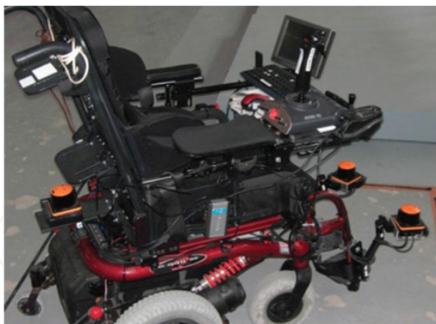
Figure 10. Assistive technology: Intelligent power wheelchair prototype for clinical applications.
