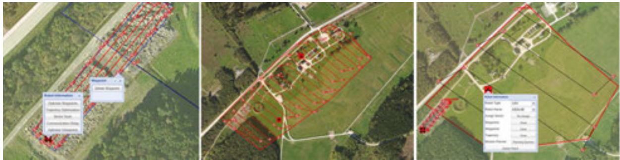
Figure 33. (i) Automated mission planning queries. (ii) Sector scan query. (iii) Optimization of waypoint query (source: ICARUS).
