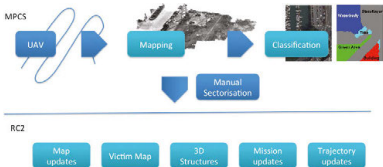
Figure 13. Concept of operations with data fusion functionalities (source: ICARUS).
