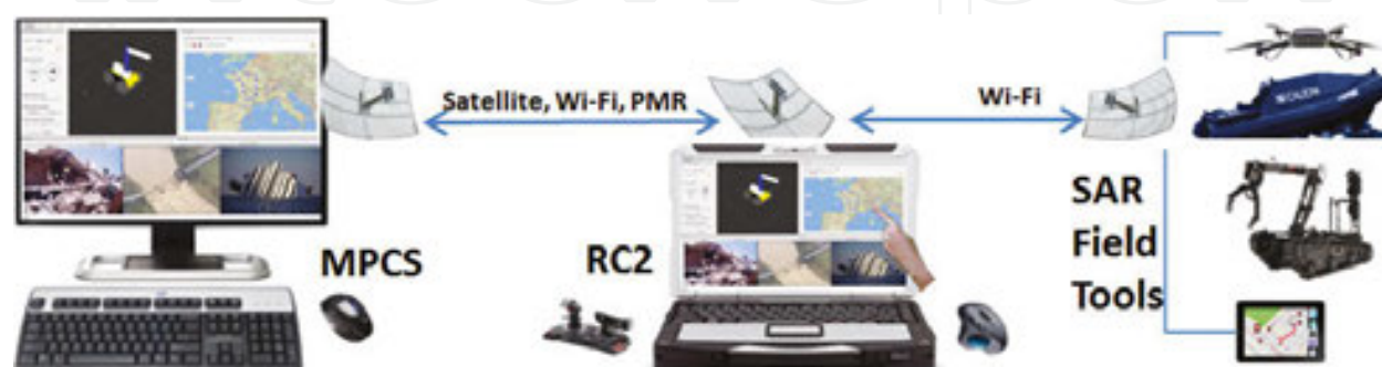
Figure 1. C2I deployment and communication framework (source: ICARUS).
