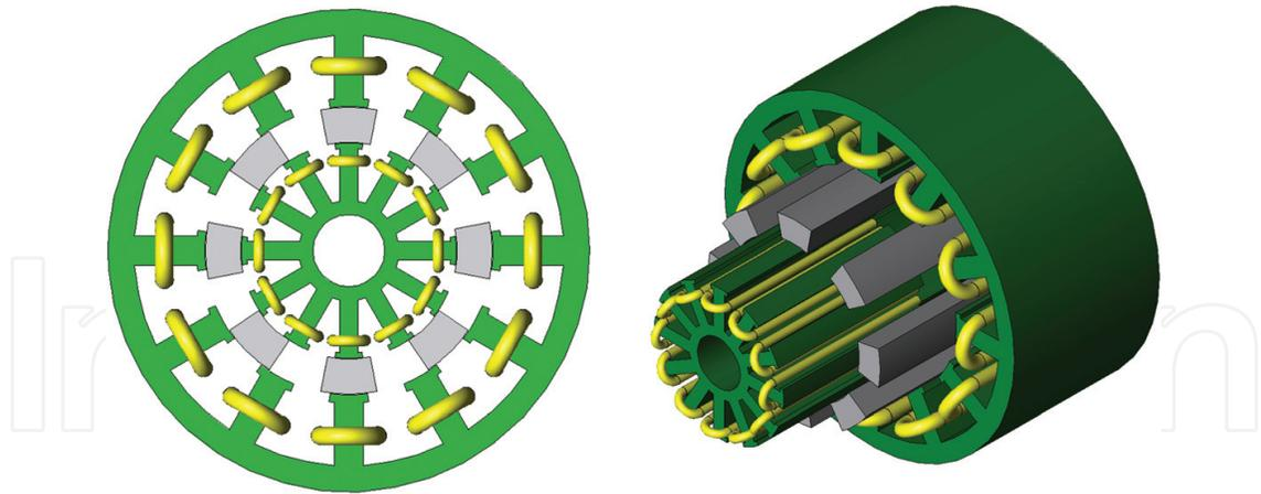
**Figure 7.** Three-phase 12/8-pole double-stator switched reluctance motor.
