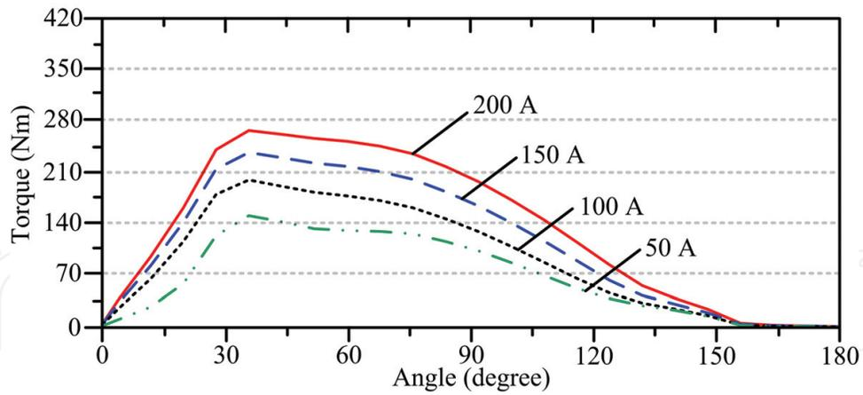
Figure 13. Torque capabilities of the switched reluctance motor.
