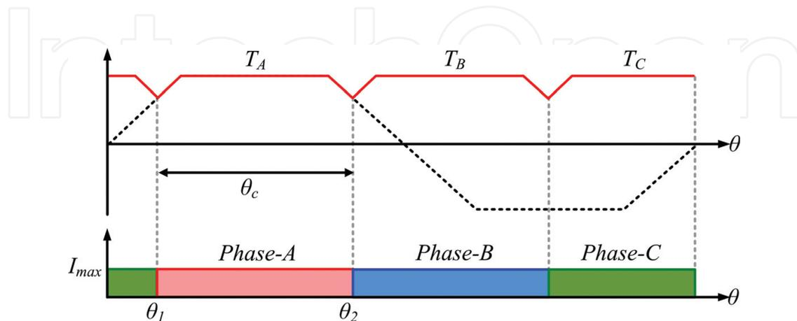
**Figure 17.** Operating principle for switched reluctance motor.
