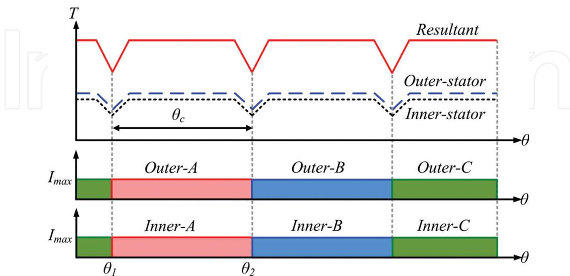
**Figure 18.** Operating principle for conventional double-stator switched reluctance motor.
