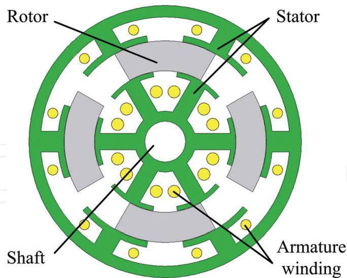
**Figure 5.** Three-phase 6/4-pole double-stator switched reluctance motor.
