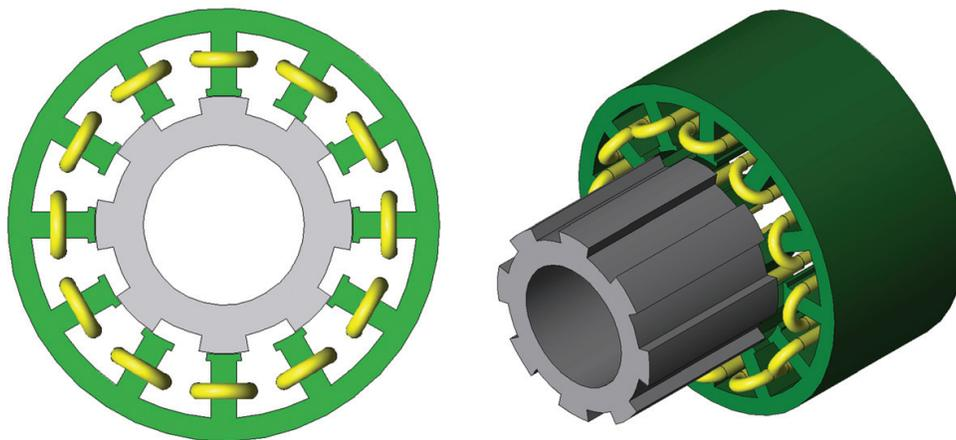
**Figure 6.** Three-phase 12/8-pole single-stator switched reluctance motor.
