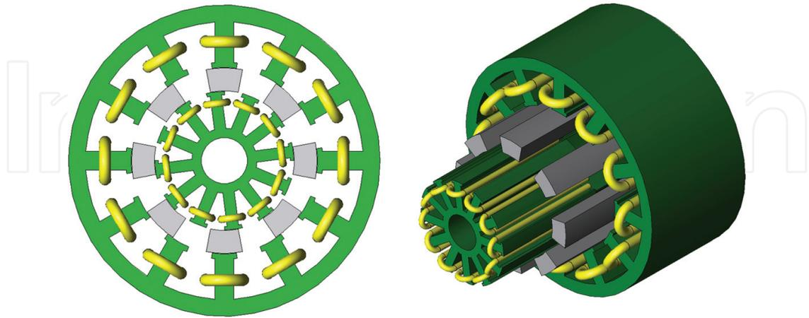
Figure 20. Three-phase 12/8-pole mechanical-offset double-stator switched reluctance motor.
