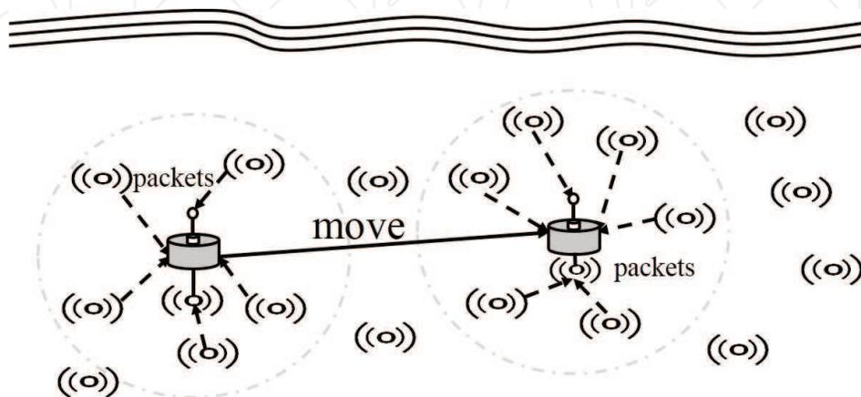
Figure 2. A mobile single-sink-based UASN.
