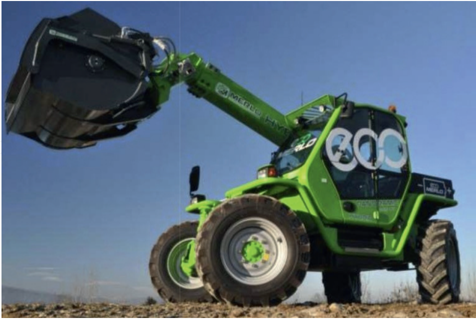
Figure 11. View of Merlo – TF 40.7 hybrid the hybrid telehandler [106].
