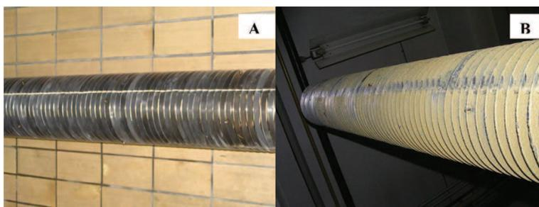
**Figure 3.** O-shaped rings before (A) and after (B) biofilm formation in HRTB.
