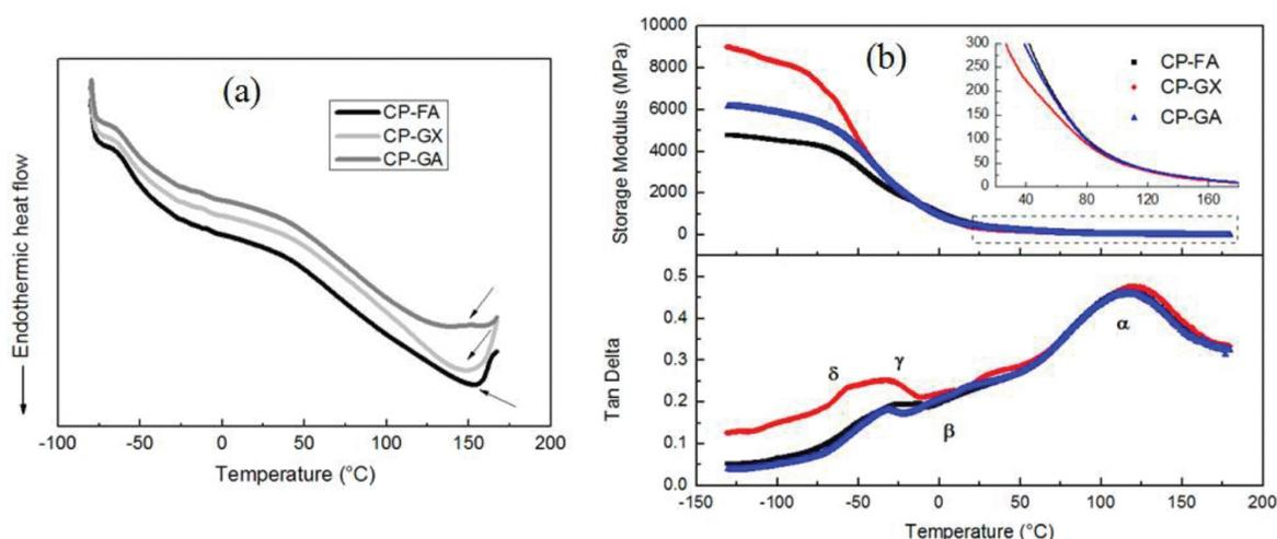
**Figure 10.** DSC (a) and DMA (b) thermograms of the aldehyde cross-linked CP-FA, CP-GX and CP-GA CPBs. The temperatures marked in DSC curves indicate the  $T_d$ . Inset is the enlarged plots marked by dashed rectangle [20]. Reproduced with permission from The Royal Society of Chemistry (2014).
