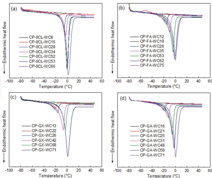
**Figure 11.** DSC thermograms showing the change in enthalpy and peak fusion temperature of the CPBs with respect to water content (WC, %). (a) CP-0CL, (b) CP-FA, (c) CP-GX and (d) CP-GA series [20]. Reproduced with permission from The Royal Society of Chemistry (2014).
