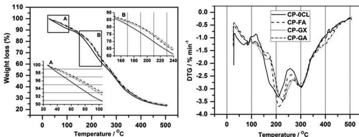
**Figure 9.** Weight loss and DTG curves of the CPBs as a function of temperature. Inset graphs denote the first stage (A) and second stage (B) of the CPB weight loss [15]. Reproduced with permission from The Royal Society of Chemistry (2012).
