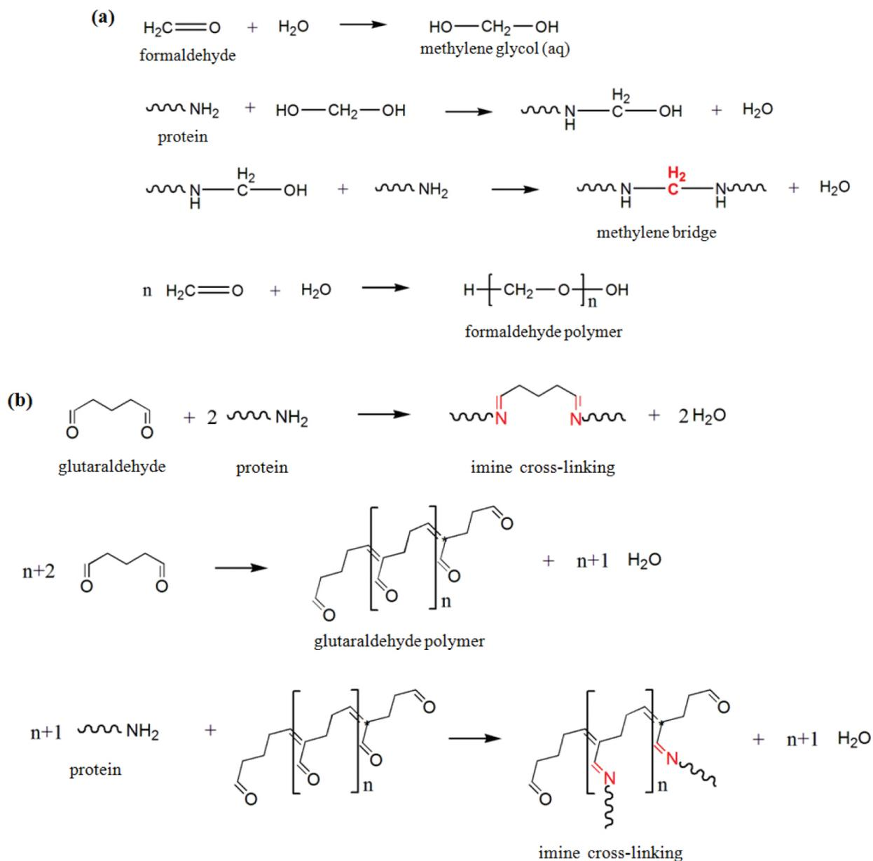
**Figure 3.** Cross-linking reactions of protein macromolecules with formaldehyde (a) showing the formation of methylene bridge and glutaraldehyde monomer/polymer, and (b) creating imine covalent bonds.
