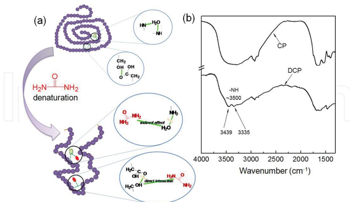
**Figure 2.** (a) Schematic illustration of the urea-induced CP denaturation via indirect and direct interactions and (b) FTIR spectra of pristine and denatured CP [15]. Reproduced with permission from The Royal Society of Chemistry (2012).
