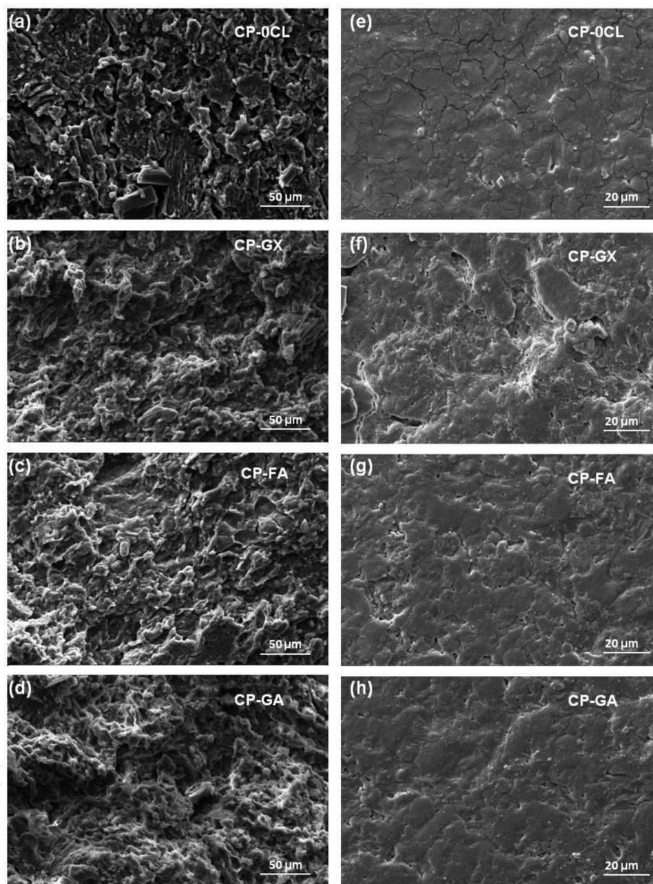
**Figure 4.** SEM images of the fractured microstructure (a–d) and the surface morphology (e–h) of the CPBs (CP-0CL, CP-FA, CP-GX and CP-GA, respectively) [15]. Reproduced with permission from The Royal Society of Chemistry (2012).
