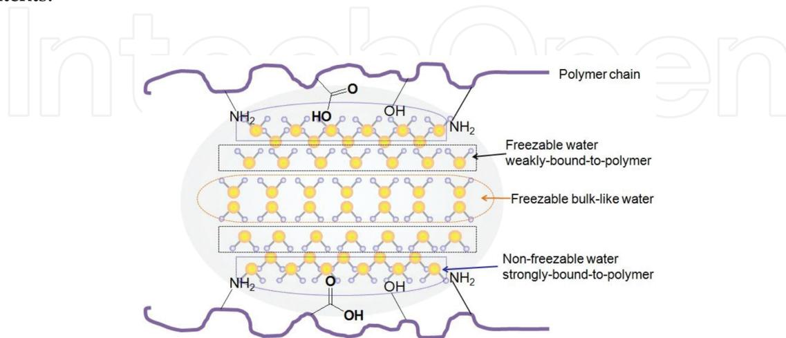
**Figure 12.** Schematic of CPB polymer chains affinity to water molecules, illustrating the presence of different states of water: freezable bulk-like water, freezable and non-freezable bound-to-polymer water [20]. Reproduced with permission from The Royal Society of Chemistry (2014).
