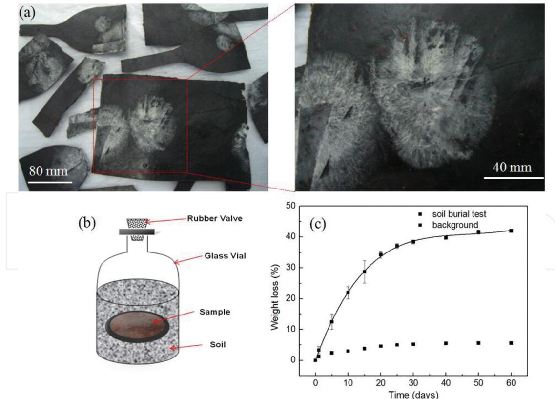
**Figure 8.** Biodegradability test of the CPB bioplastics. (a) Microbial fungi growth after 6 months under natural-storage condition (at room temperature and 40 RH%); (b) schematic of soil-burial test and (c) results of weight loss (%) of the bioplastics measured by soil-burial test referenced with a background.
