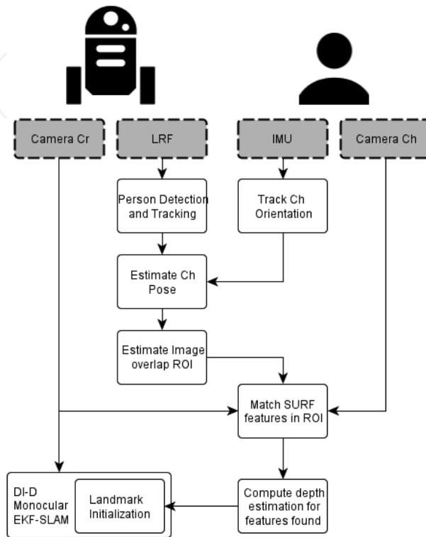
**Figure 4.** Block diagram of the final implementation, with sensors on gray boxes and software processes on clear blocks. The updated landmark initialization is one of the cornerstone processes in any feature-based EKF-SLAM technique.
