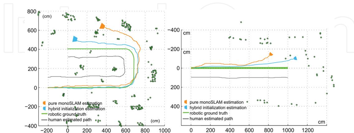
**Figure 7.** Trajectories estimated with classical DI-D monocular SLAM (orange plots) and with the new non-constant stereo DI-D approach for feature initialization (blue plots). Green line denotes robot ground truth; gray line denotes  $C_h$  ground truth.
