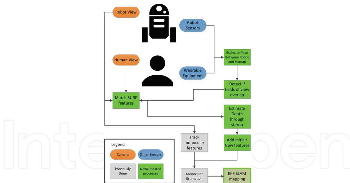
**Figure 1.** DI-D monocular EKF-SLAM components within human-robot collaborative.
