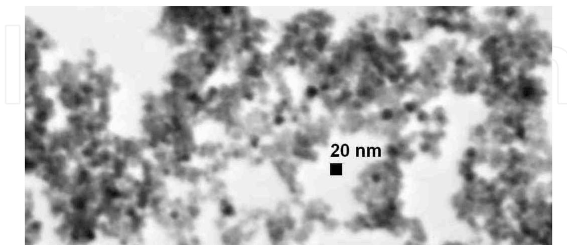
**Figure 1.** TEM picture of 0.5% Mn-doped ZnO NPs, where they are seen with strong black color, with spherical morphology and uniform size. The gray background is produced by the human albumin used to disperse the particles.
