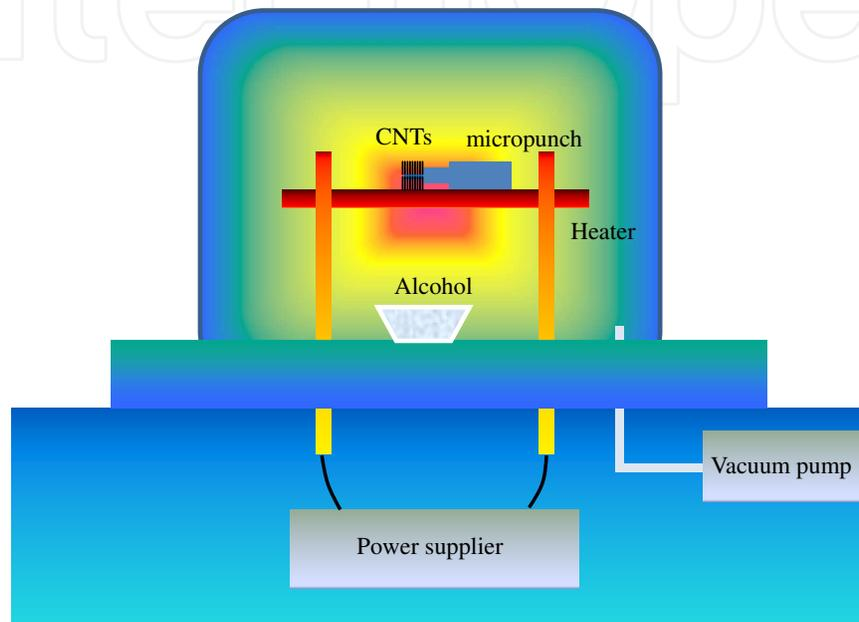
**Figure 2.** Equipment for CNTs synthesis
