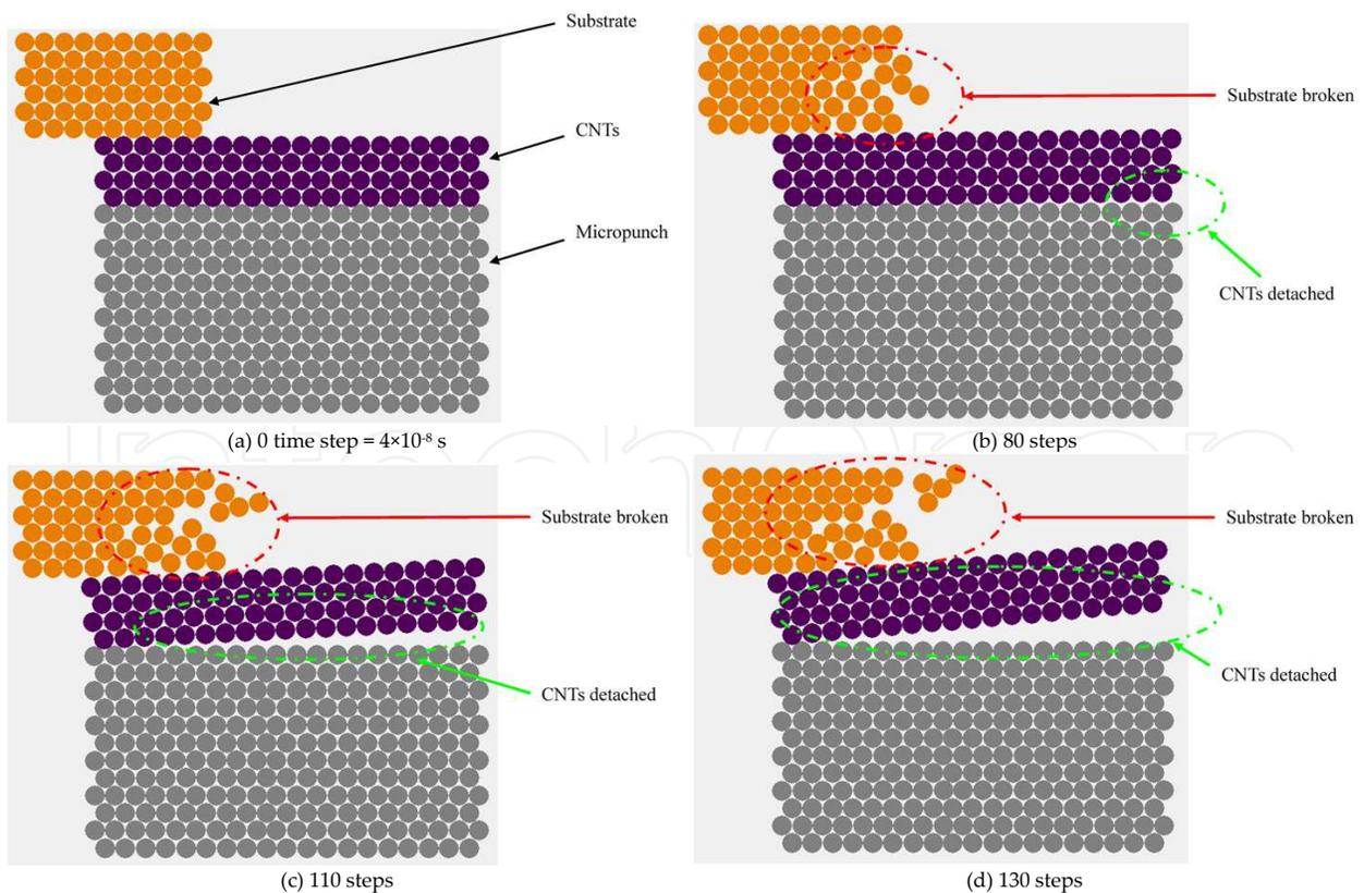
**Figure 9.** MCA simulation of micropunching with CNTs coating
