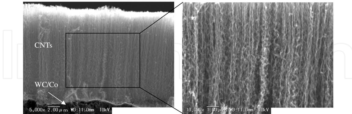
**Figure 3.** Synthesized CNTs coated on micropunch
