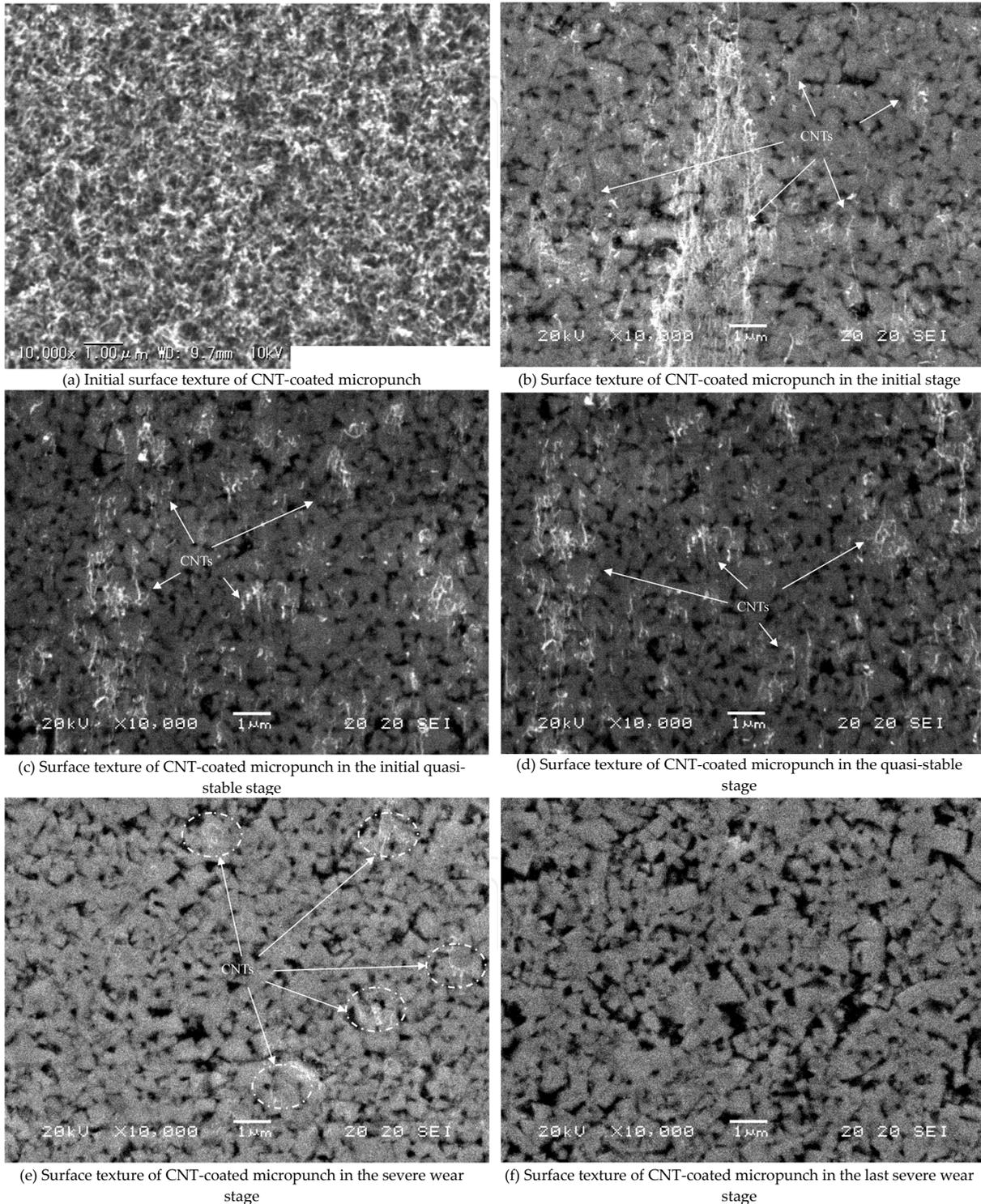
**Figure 6.** Surface texture of micropunch in various conditions
