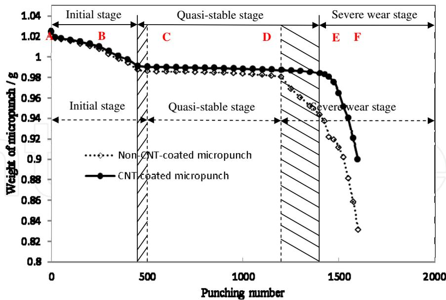
Figure 5. Relationship between wear loss and punching numbers
