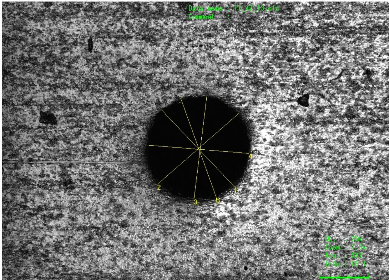
Figure 7. Profile of punched microhole measured by OLS3000
