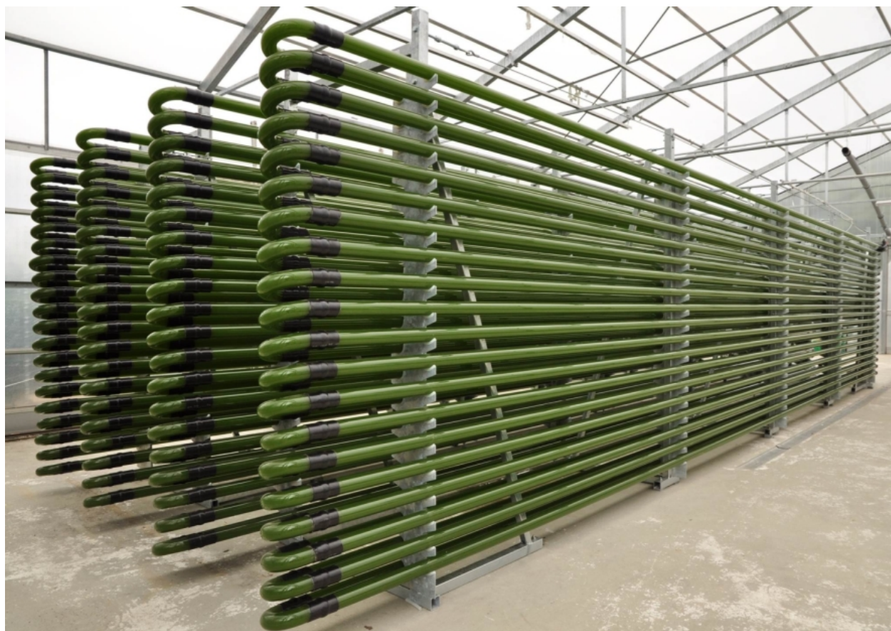
Figure 6. Photobioreactor for large scale algae production [122]
