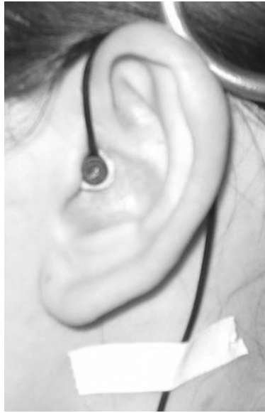
Figure 3. Blocked-ear-canal measurement with miniature microphone
