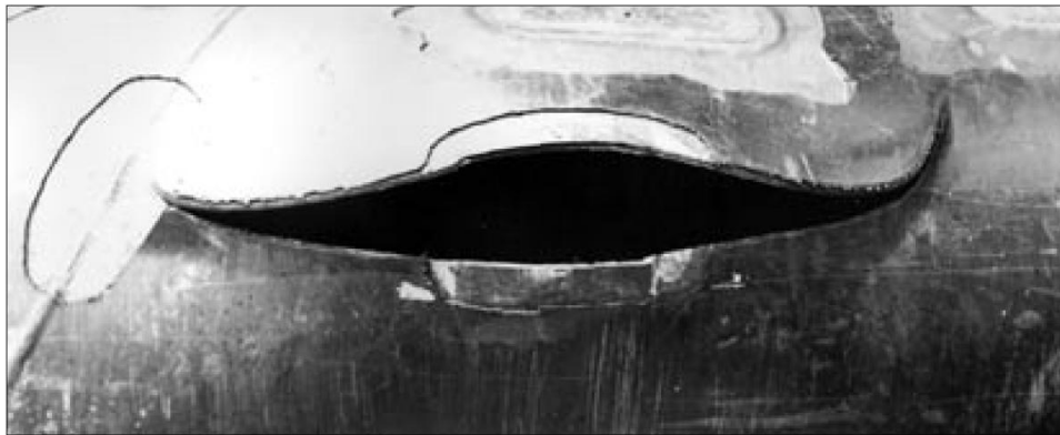
Figure 17. Burst initiated on slit B – a detail
