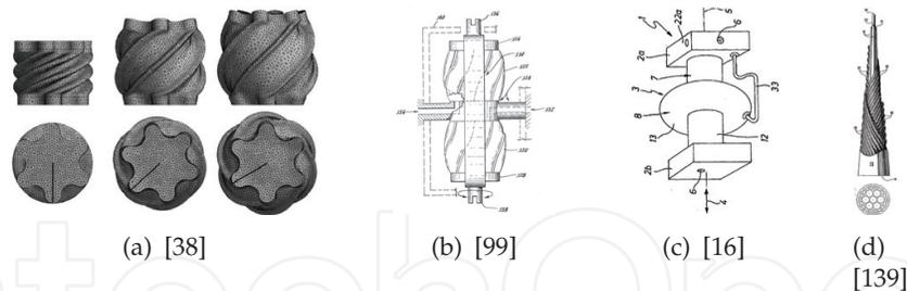
**Figure 7.** Actuators with two directions of motion
