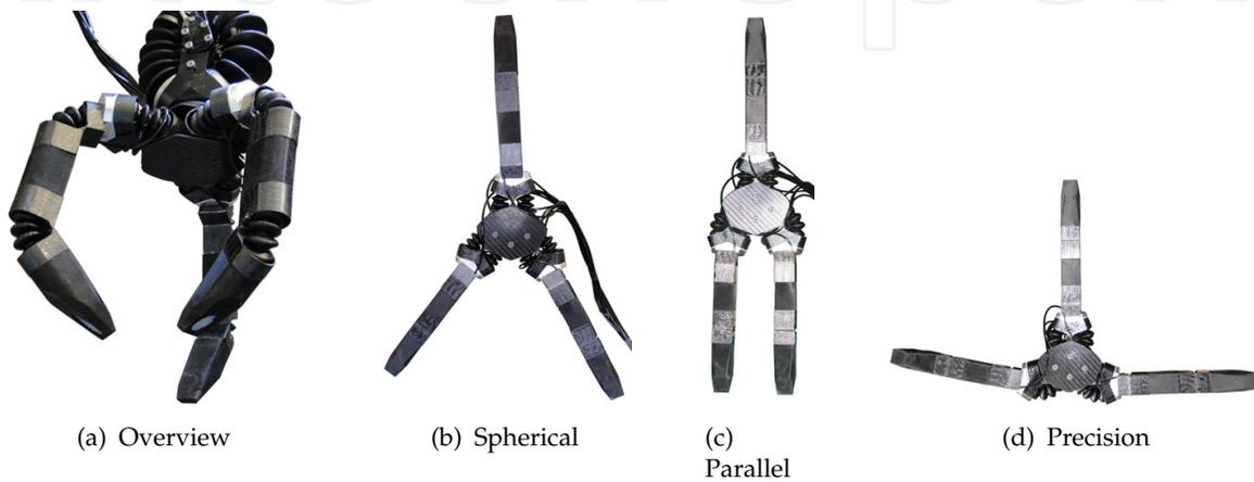
**Figure 35.** Main Base Positions of the Composite Gripper
