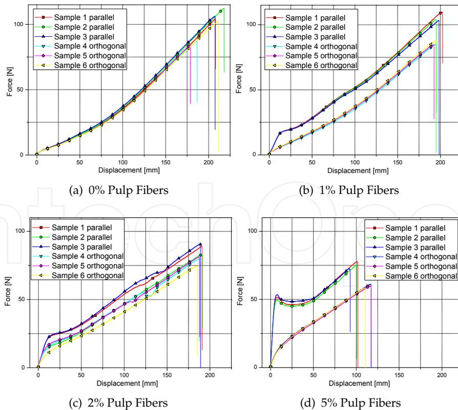
**Figure 14.** Force-Displacement Plots for different Pulp Fiber Concentrations
