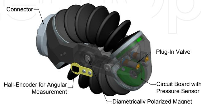
**Figure 31.** Highly Integrated Flexible Fluidic Drive Module
