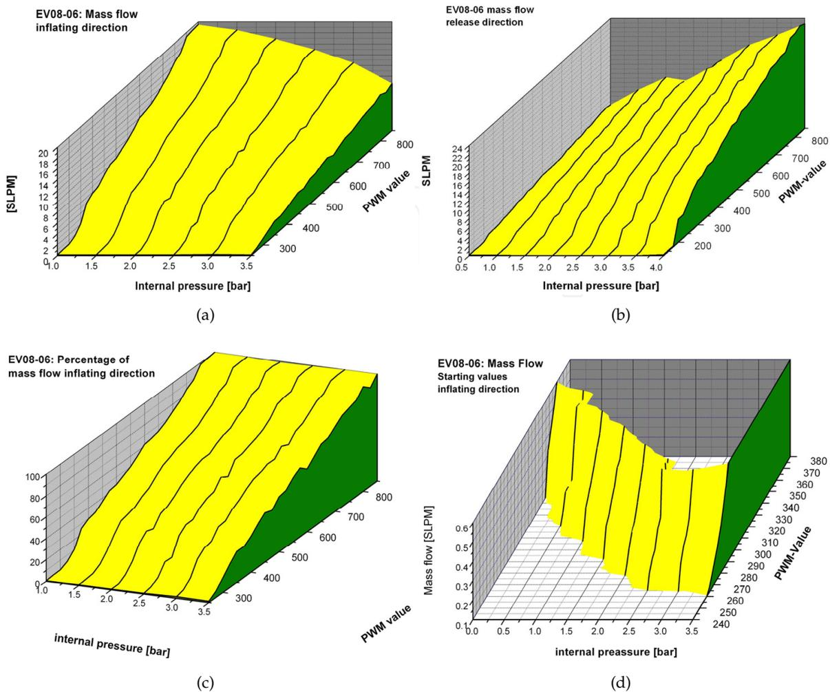
**Figure 25.** Flow Characteristics of an EV08-Switching Valve
