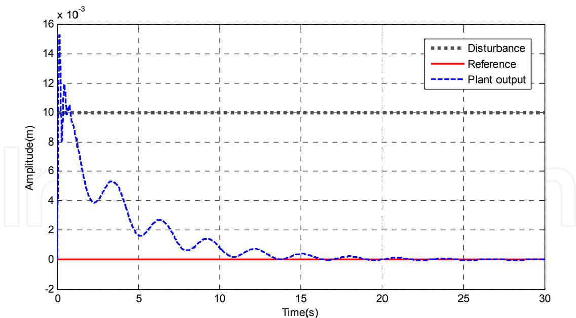
**Figure 4.** Non-controlled system response to a step disturbance
