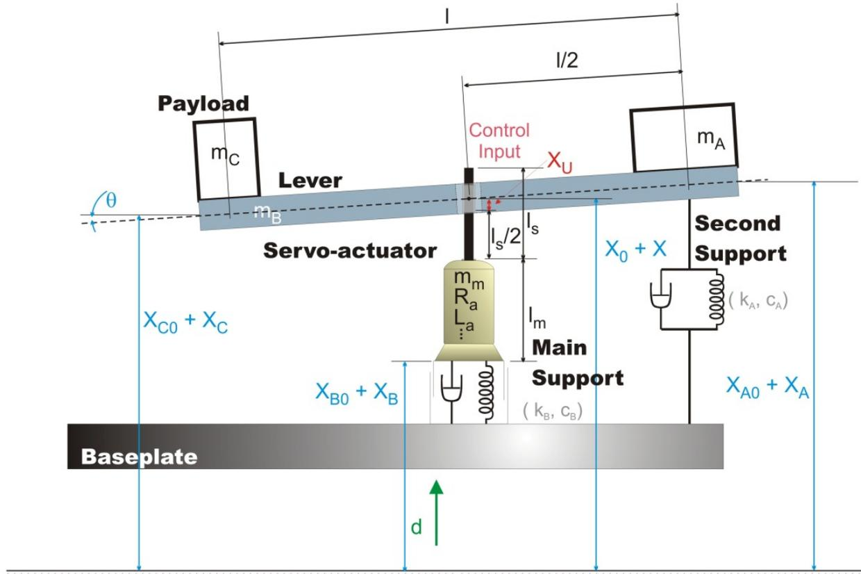
**Figure 2.** Electromechanical system
