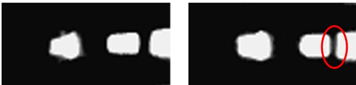
Figure 25. An example for the tiny differences between the images containing correct and faulty components
