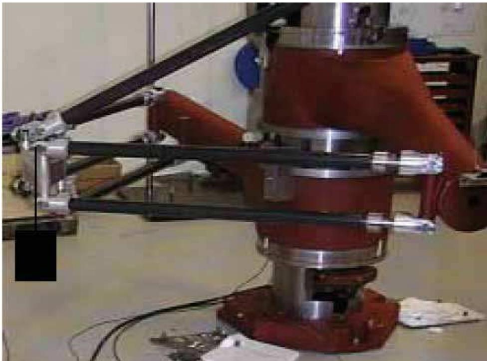
Figure 24. Setup of the TAU robot's Stiffness Measurement
