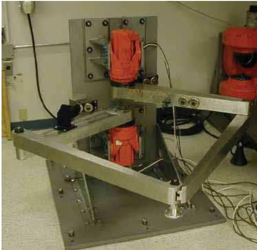
Figure 14. Two-Arm Test Platform (double SCARA structure)
