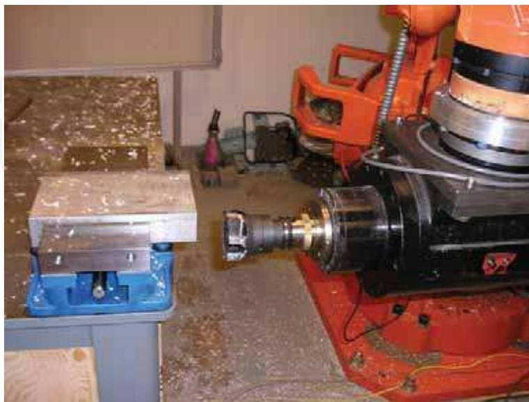
Figure 26. Robotic Milling Setup
