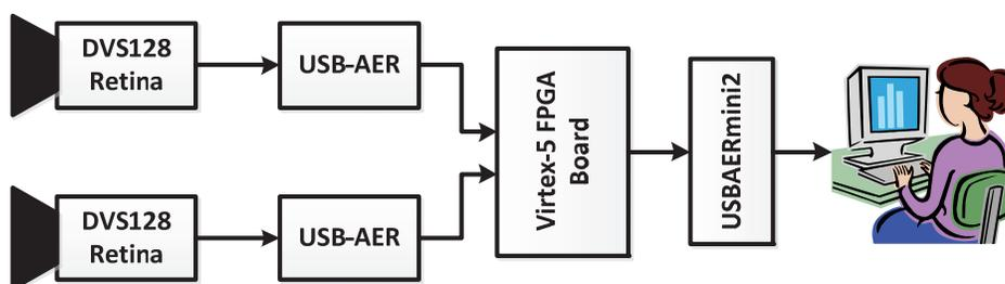
**Figure 10.** Complete system with all the elements used
