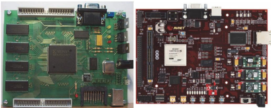
**Figure 11.** Left, USB-AER board; right, Virtex-5 FPGA board.
