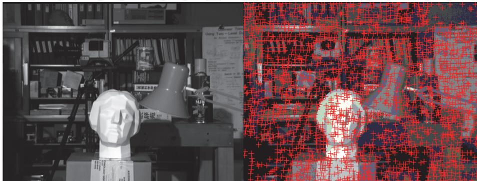
**Figure 8.** Edge detections in a features-based algorithm.
