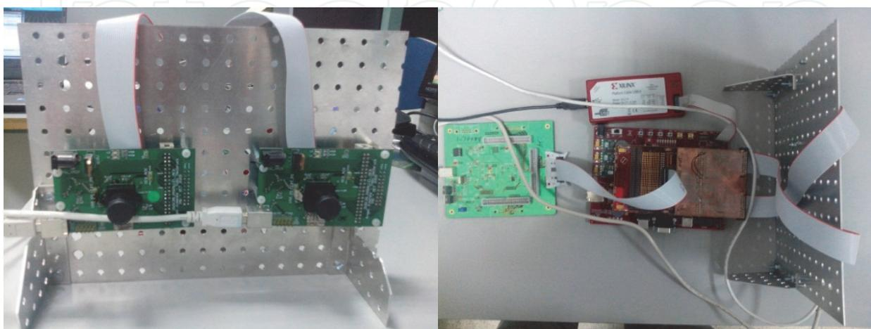
**Figure 12.** Virtex-5 with AER retinas and USB AERmini2.
