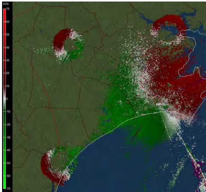
Fig. 19. Field of velocities obtained from the radar at Moorhead City, NC, on July 27, 2011 at 5:08 in the morning. The color bar indicates categories in kts; red away from the radar and green is toward. Elevation is 0.5°.
