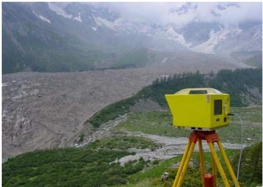
Fig. 4. The Optech ILRIS-3D laser scanner during a field masurements (photo P. Federici)
