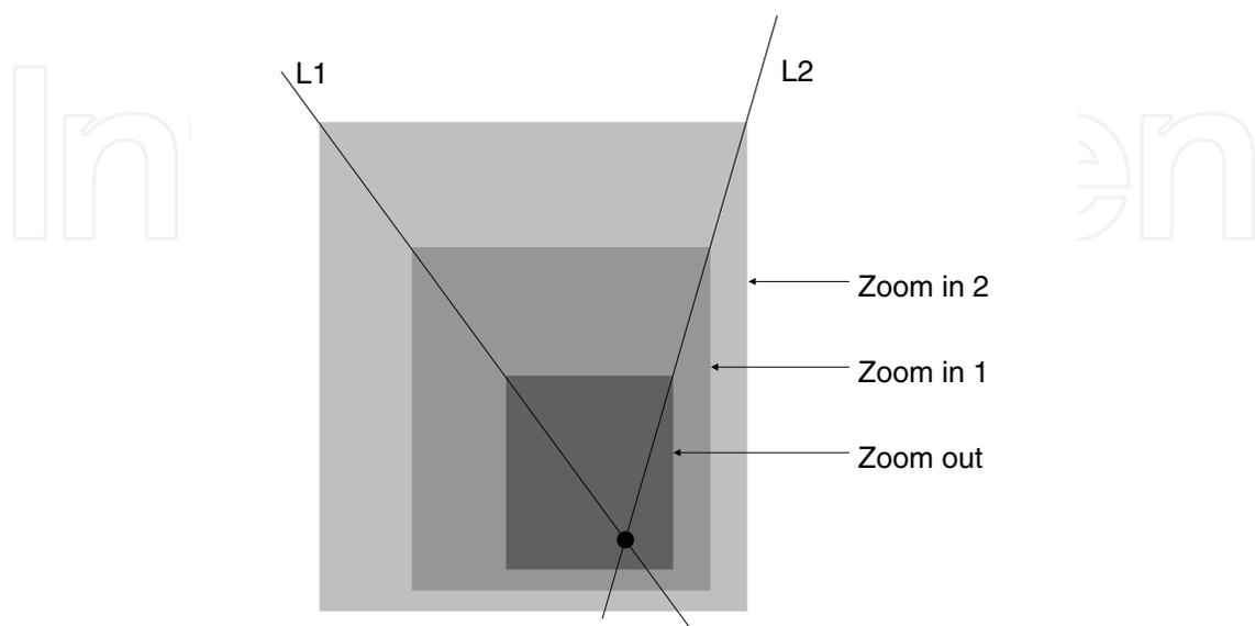
Fig. 4. Geometric determination of the image centre by using zoomed images. The intersection of the lines  $L1$  and  $L2$ , defined by the tracing of two points across the zoomed images, corresponds with the image centre.
