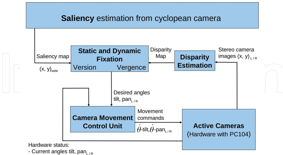
Fig. 5. Angular-position control scheme of the trinocular system.
