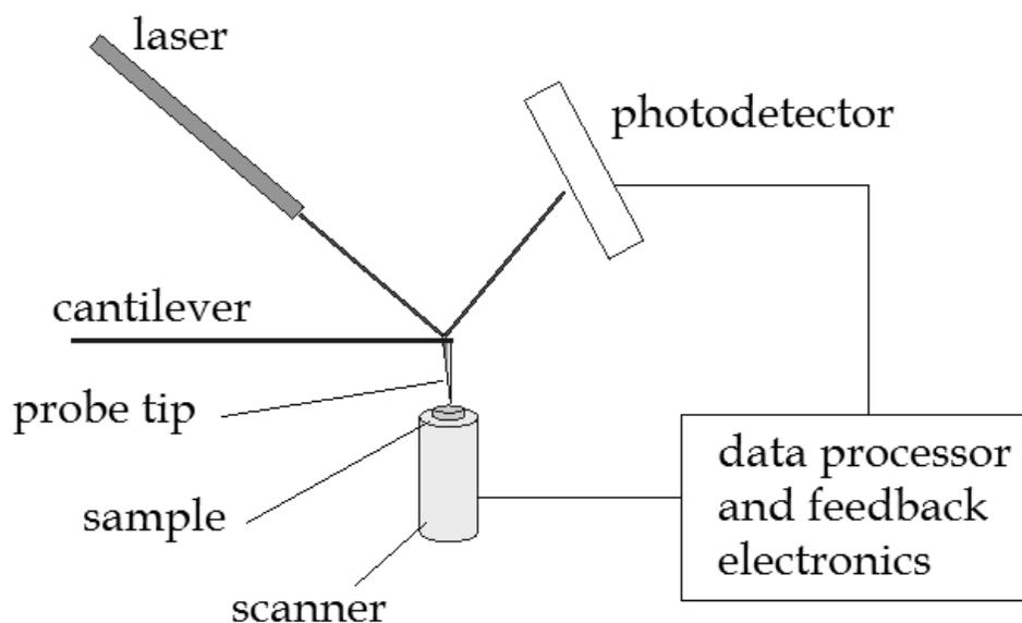
Fig. 1. Principle of AFM.
