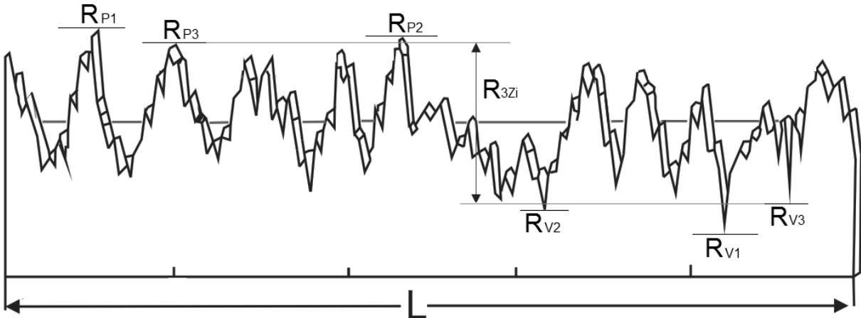
Fig. 16. The two highest peaks ( $R_{P1}$  and  $R_{P2}$ ) and the two deepest valleys ( $R_{V1}$  and  $R_{V2}$ ) are disregarded. The  $R_{3zi}$  is counted from the third highest peak ( $R_{P3}$ ) and the third deepest valley ( $R_{V3}$ ) (adapted from Predev, 2011).
