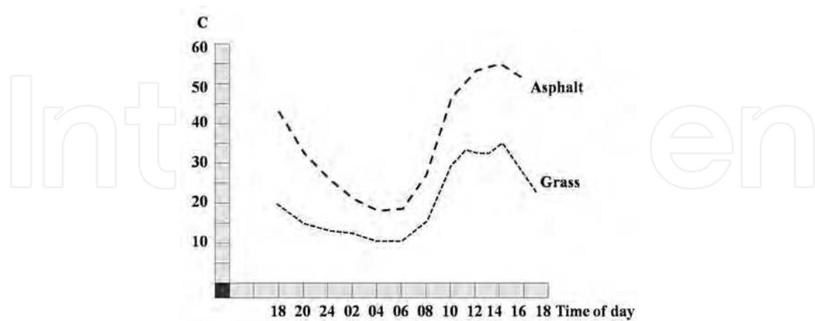
Fig. 3. Earth Surface temperature through 24 hour ( Source : Amjad Almusaed 2010)
