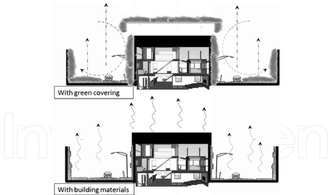
Fig. 4. The comportment of different surfaces (green covering - non green covering)
