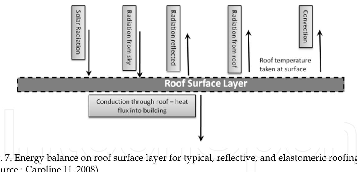
Fig. 7. Energy balance on roof surface layer for typical, reflective, and elastomeric roofing (Source : Caroline H. 2008)
